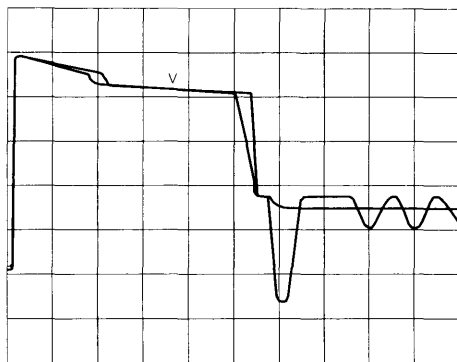
Figure 22 : Effect of the Resistor in Parallel connected to the yoke. V = 10V/div.
