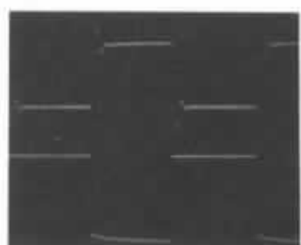
100 Hz variation courant shunt. 5 V/cm
