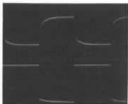
100 Hz variation de courant shunt. 5 V/cm
