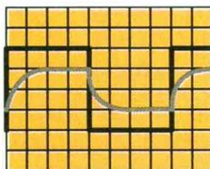
$R_1 C_1 < R_2 C_2$
