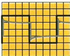
$R_1 C_1 > R_2 C_2$
