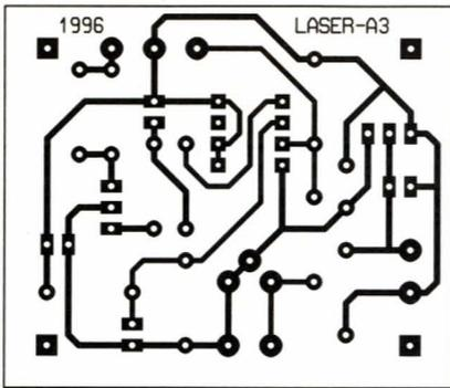
**4/5** CIRCUIT IMPRIMÉ ET IMPLANTATION.
