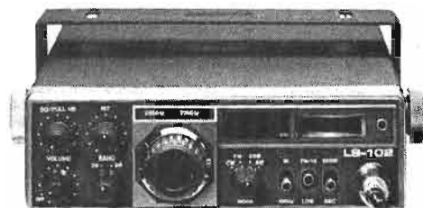
LS 102 Transceiver 10 m, tous modes FM / AM / SSB / CW, 10 W HF 12 V
