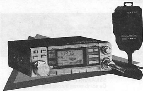
FT 270R Transceiver 144 MHz, FM, 25 W, 13,8 V
