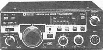
transceiver 144 MHz FM-USB-LSB-CW 12 V-25 W Prix : 4950 F
