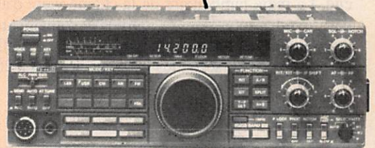
TS 440 SP SSB-AM-FM-RTTY 100 KHz-30 MHz-100 W HF
