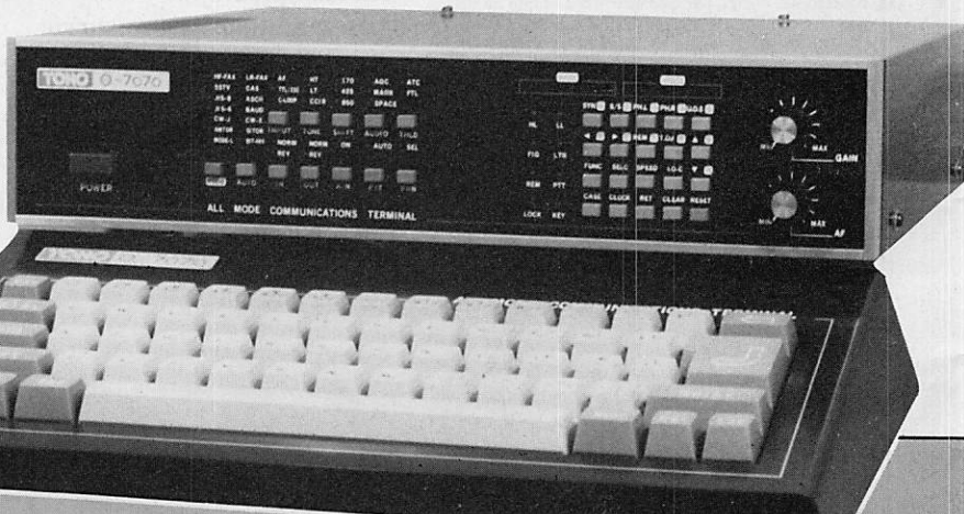
TONO 7070 – Terminal de commu- nication tous modes : CW, RTTY (Baudot, ASCII et JIS), AMTOR, SSTV, FAX.
