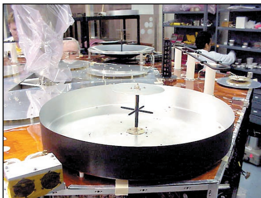
Antenne back-fire 1,2 GHz (Fourniture AMSAT-France).
