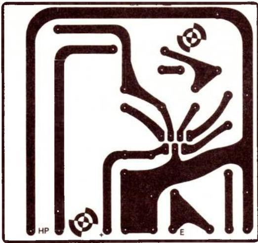
Figure 4 - Circuit imprimé ampli 10 W
