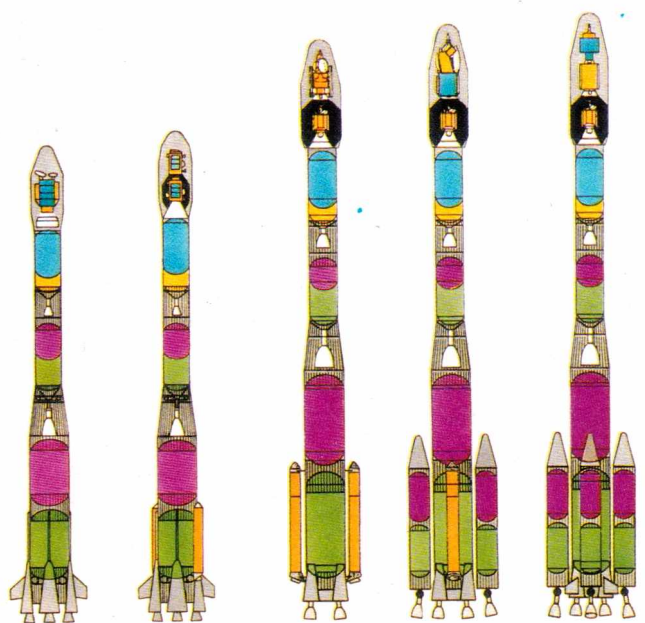
ariane 1 ariane 3 ariane 4 ariane 4 ariane 4 1750 kg* 2580 kg* 42P 2600 kg* 44LP 3700 kg* 44L 4200 kg*
